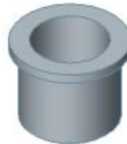
ITEM 4 BUSHING, NYLON SCALE: 4:1
