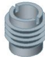
ITEM 7 THREADED INSERT SCALE: 4:1
